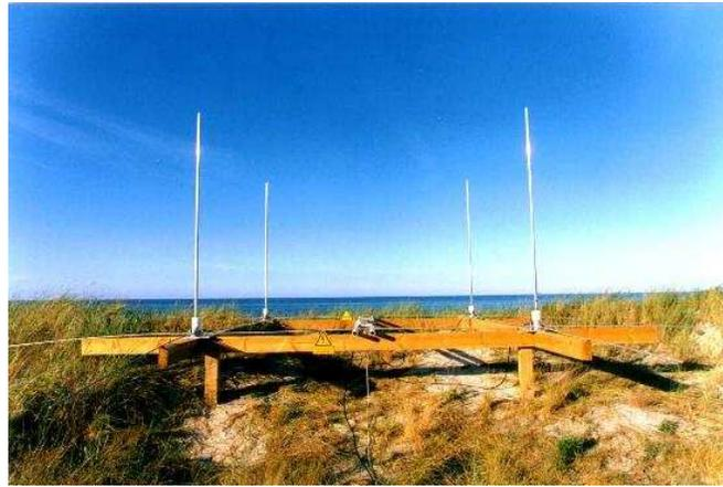
Figure 1.5: Transmitting array of a WERA radar.
