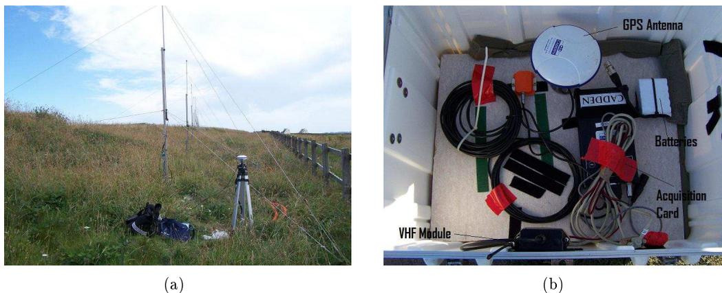
Figure 1.12: (a) Picture of the GPS base near antenna 16 (b) Picture of the GPS module in the hermetic box of the floating antenna.
