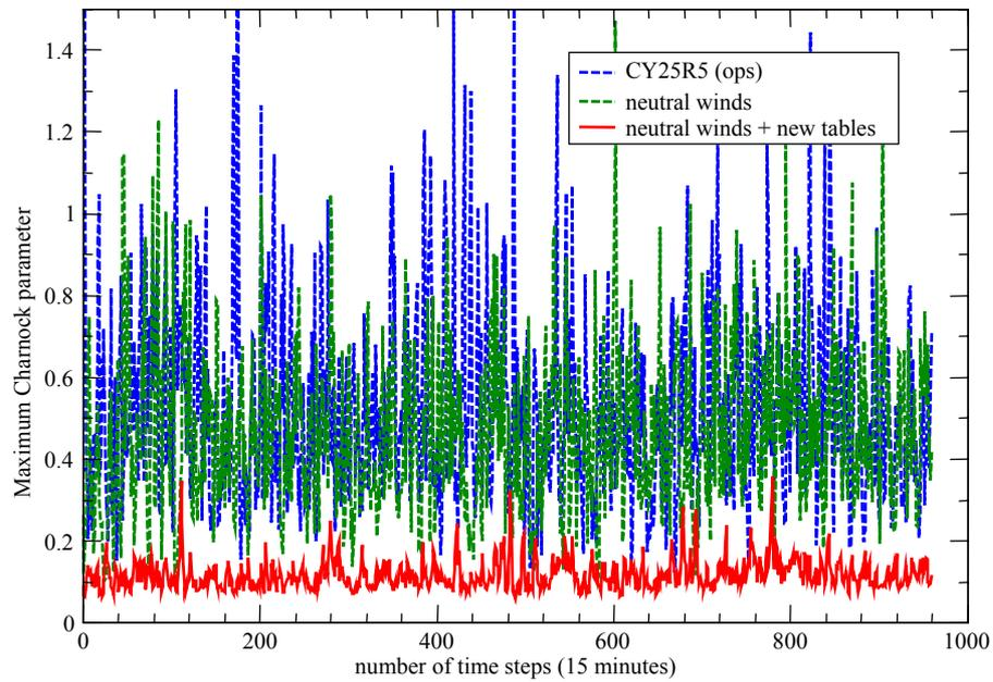
Figure 13: Maximum Charnock parameter norm as found in 10-day coupled forecast log files.
