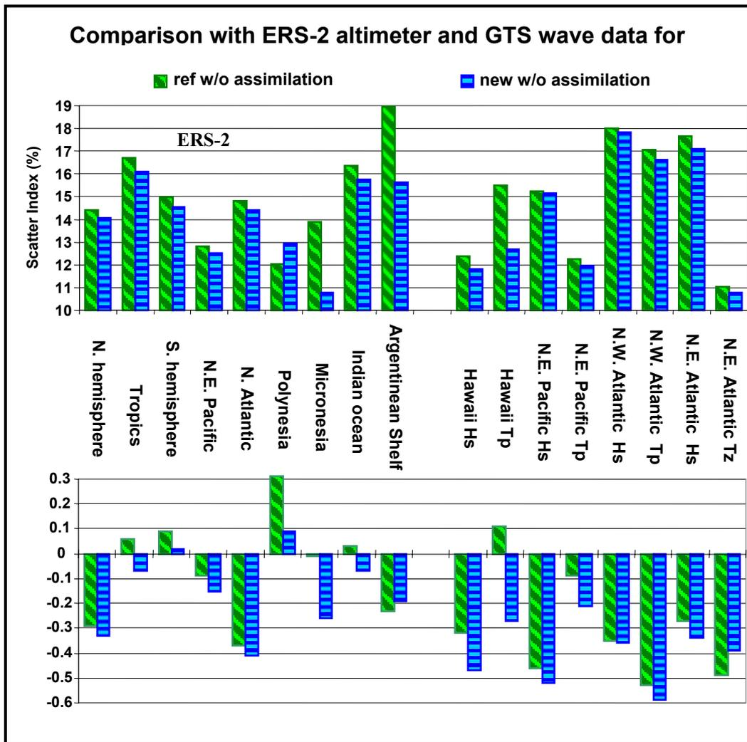
Figure 11: Same as Figure 8 and 9 combined for December 2002. Only runs without data assimilation are compared.
