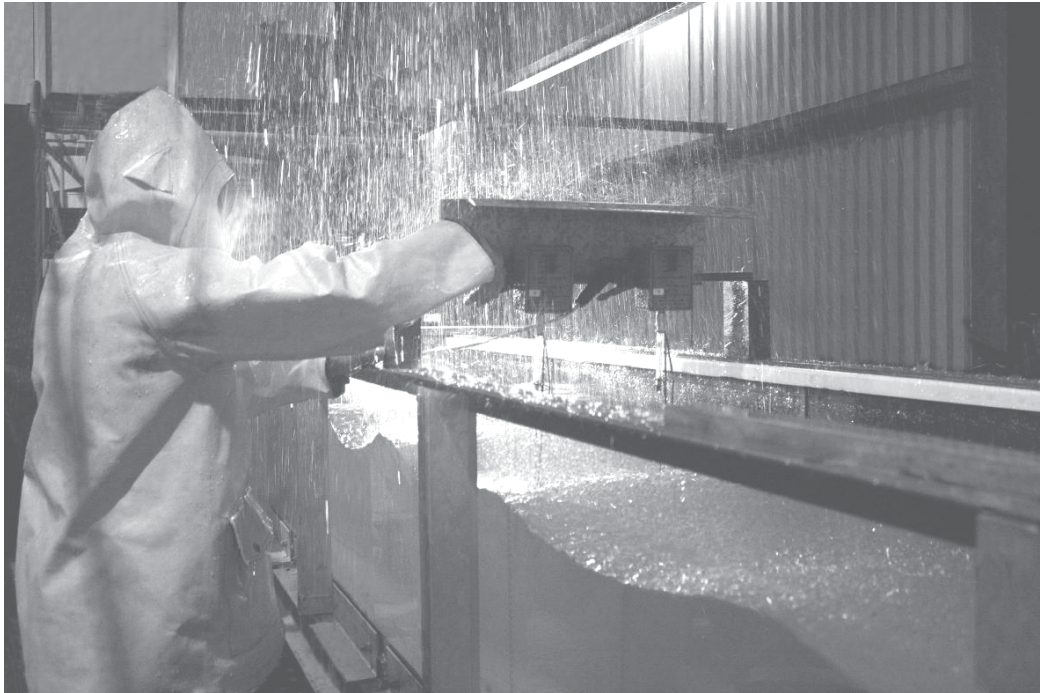
Figure 4-5. Photo during rainfall wave attenuation measurements. Note roof protecting the wave probe pair.
