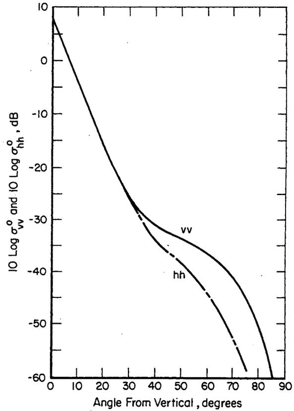
FIGURE 3. Measured average backscattering cross section per unit area of relatively calm sea surface at X band for vertical and horizontal polarization states.
