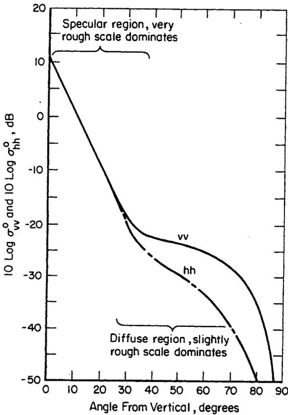
FIGURE 2. Theoretical curves for backscattering cross section per unit area of composite surface having a dielectric constant  $\epsilon_r = 5.0$  for vertical and horizontal polarization states.
