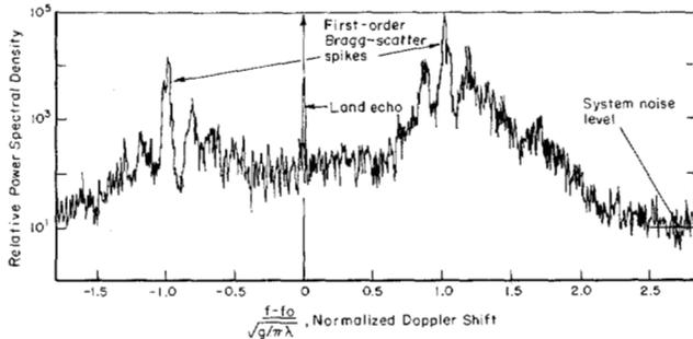
Fig. 1. Sea echo Doppler spectrum at 30 MHz for near-grazing backscatter, vertical polarization: January 25, 1972 [After Tyler, et. al., 10].
