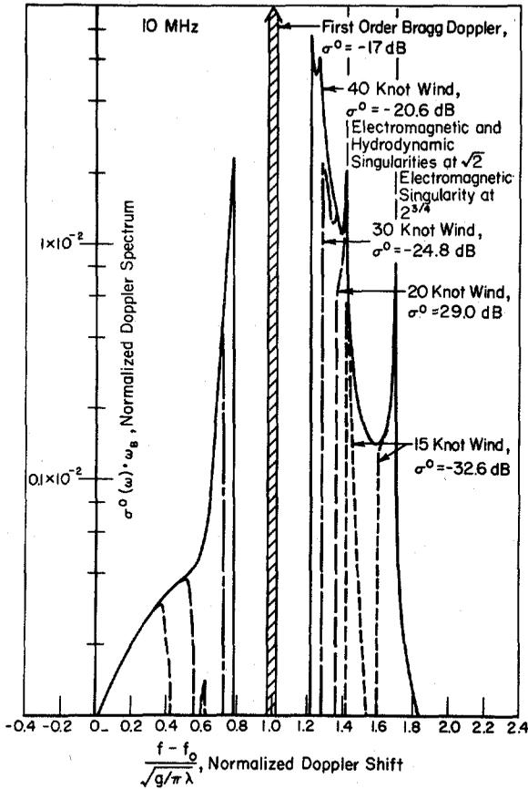
Fig. 3. Predicted Doppler spectrum of first and second-order near-grazing sea backscatter at 10 MHz for propagation in upwind direction (Phillips semi-isotropic waveheight spectrum assumed).
