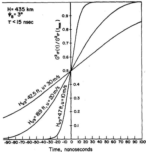
Fig. 5. Leading edge of averaged altimeter output versus time predicted for pulse-limited operation.
