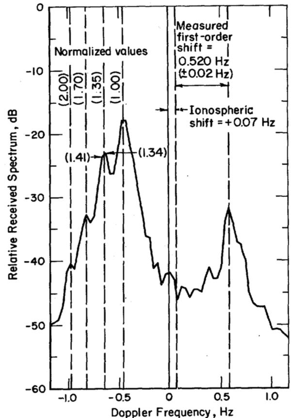
Fig. 2. Sea echo Doppler spectrum at 25.75 MHz for ionospherically propagated backscatter: March 30, 1971 [After Barnum, see [2]].
