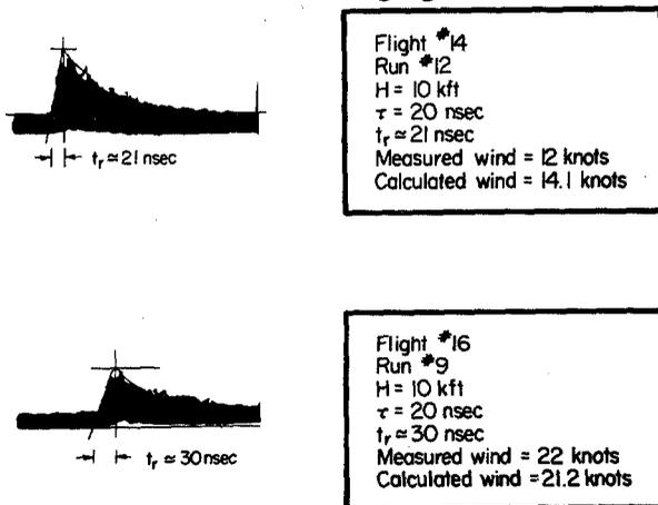
Fig. 6. Measured aircraft altimeter responses. Wind speeds inferred from rise times are compared to observed wind speeds.
