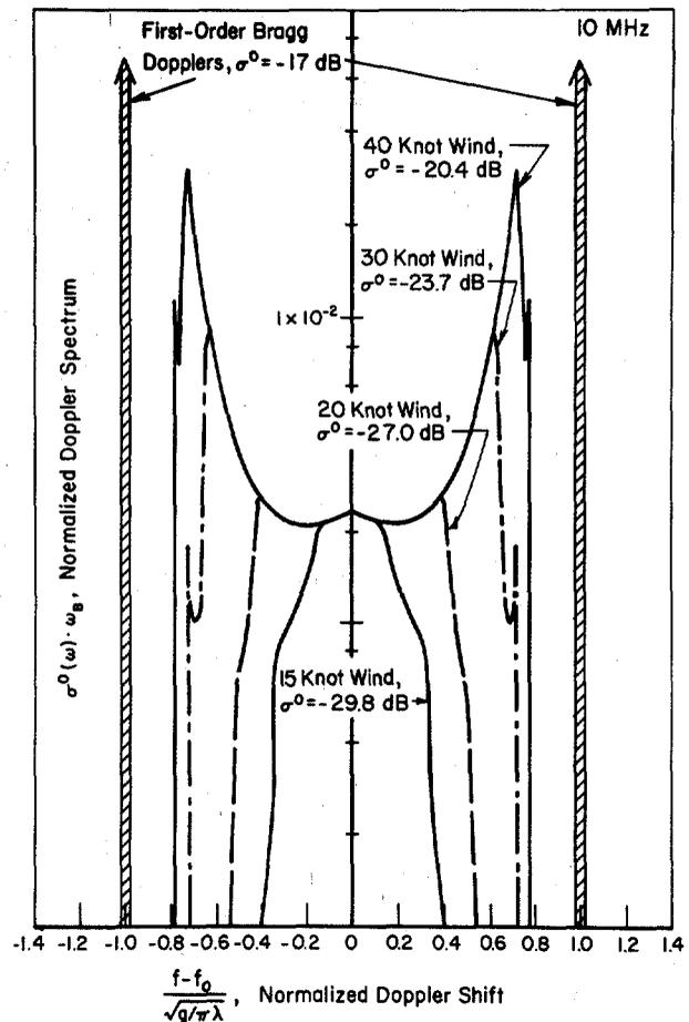
Fig. 4. Predicted Doppler spectrum of first and second-order near-grazing sea backscatter at 10 MHz for propagation in crosswind direction (Phillips semi-isotropic waveheight spectrum assumed).
