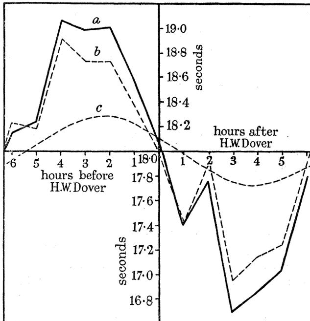
FIGURE 6. Estimated values of apparent period of waves originally of 18 sec. period which travel across the continental shelf in a direction  $035^\circ$  as in figure 3, and arrive at Perranporth at various tidal times. *a*, total value; *b*, effect of tidal stream velocities; *c*, effect of changing water depth in tides.
