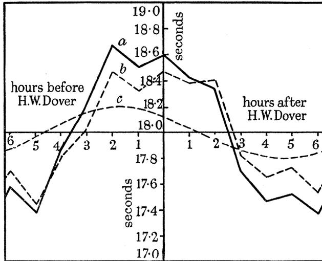
FIGURE 7. Estimated values of apparent period of waves originally of 18 sec. period which travel across the continental shelf in a direction  $090^\circ$  and arrive at Perranporth at various tidal times. *a*, total value; *b*, effect of tidal streams; *c*, effect of changing water depth in tides.
