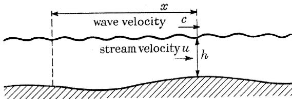
FIGURE 2. Kinematics of waves on streams (one-dimensional problem).
