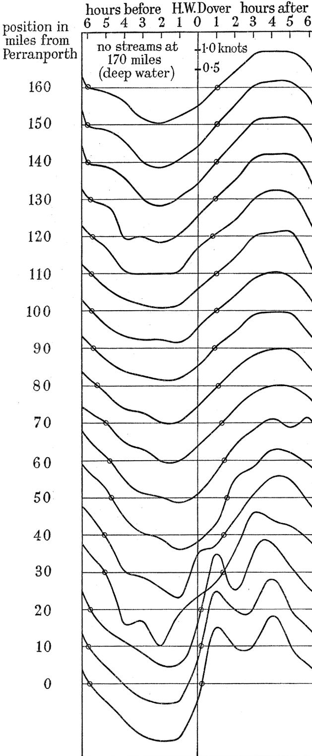
Graphs against time, of the component of velocity of tidal stream (at springs) in the direction of wave progress from Falkland Islands, past Land's End to Perranporth. The curves are based on the Admiralty charts of tidal streams issued for hourly intervals relative to high water at Dover. The horizontal lines are at intervals of 1 knot on the vertical scale. The times at which the streams are zero are indicated by small circles.
