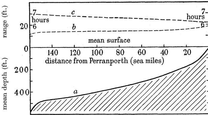
FIGURE 5. Mean depth of water at various points along the path shown in figure 3. *a*, mean depth of water; *b*, range of tide at springs; *c*, hours by which high tide precedes the time of high tide at Dover.
