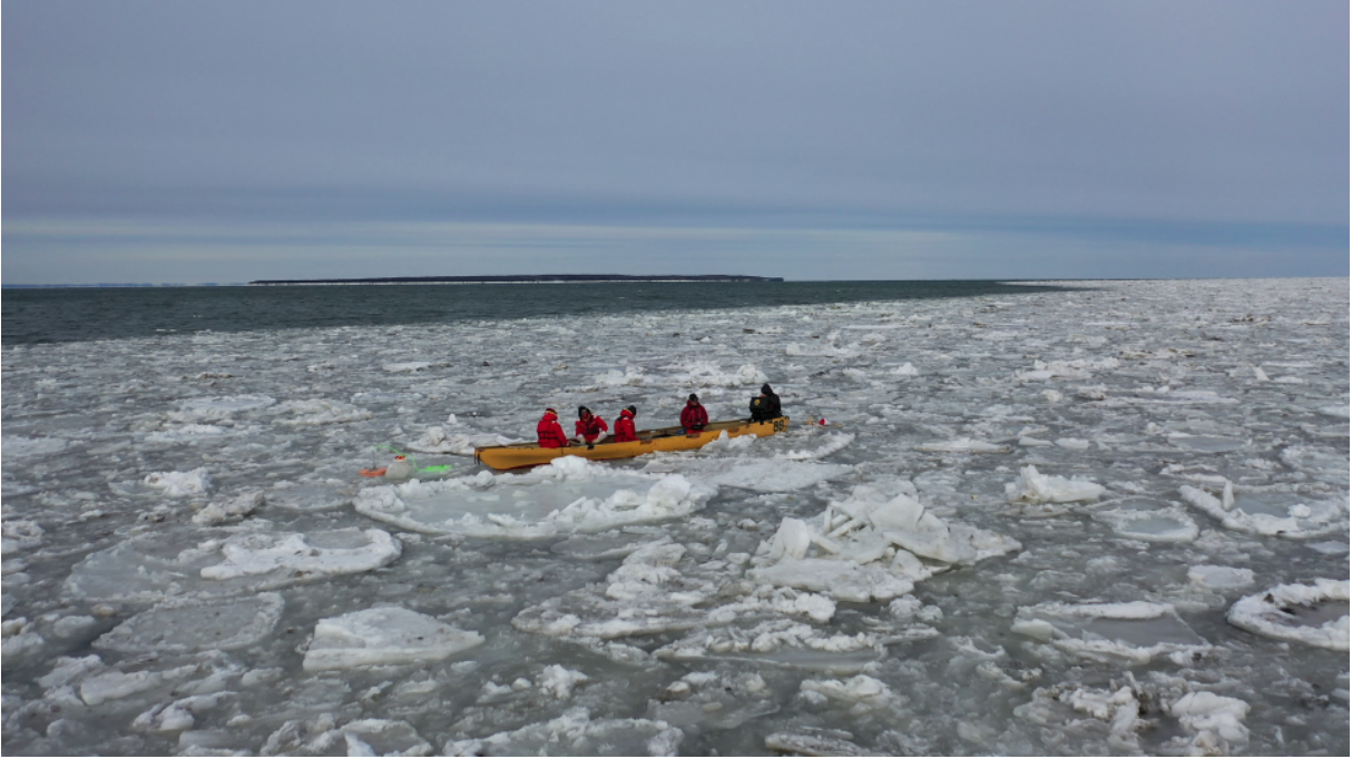
Figure 2.2 – Picture taken by a UAV facing North of the ice canoe in operation and its five-member crew during the 2020-02-13 deployment off the BdHH, with Bic Island visible in the back. The pink, red and green objects on the ice floe just to the left of the canoe are respectively the buoy of S497, a SKIB buoy, and the digital cable connecting S497 to a computer to start the data acquisition.
