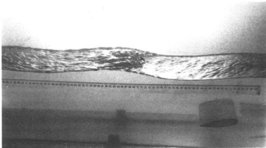
*Figure 3* Quasi-steady spilling breaker generated in a laboratory flume by the submerged hydrofoil seen at the lower right side. (M. L. Banner)
