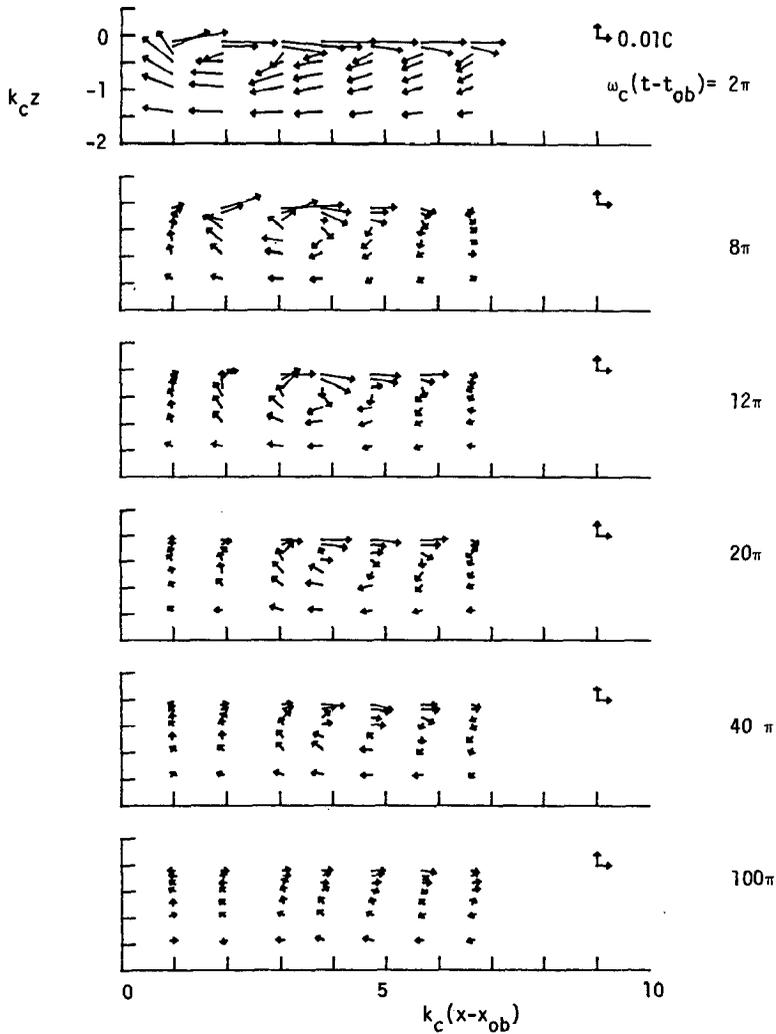
Figure 4 The mean velocity field at the following times after a plunging breaker occurs (from top to bottom at 1, 4, 6, 10, 20, and 50 periods); from Rapp & Melville (1990) with permission of The Royal Society, London.
