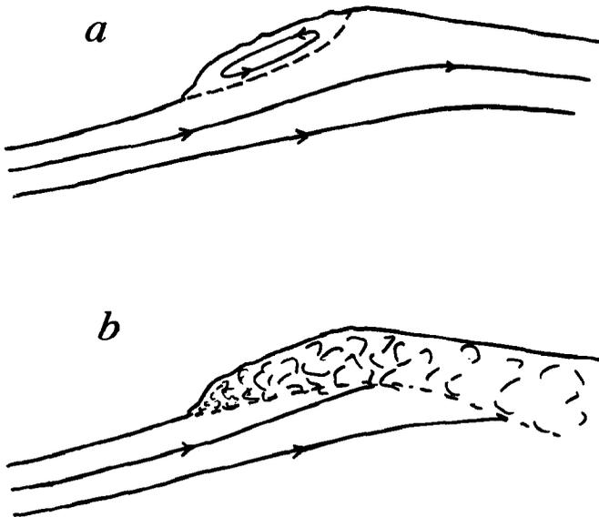
Figure 5 Spilling breakers: (a) The traditional view with a surface “roller,” (b) viewed as the source of a turbulent region.
