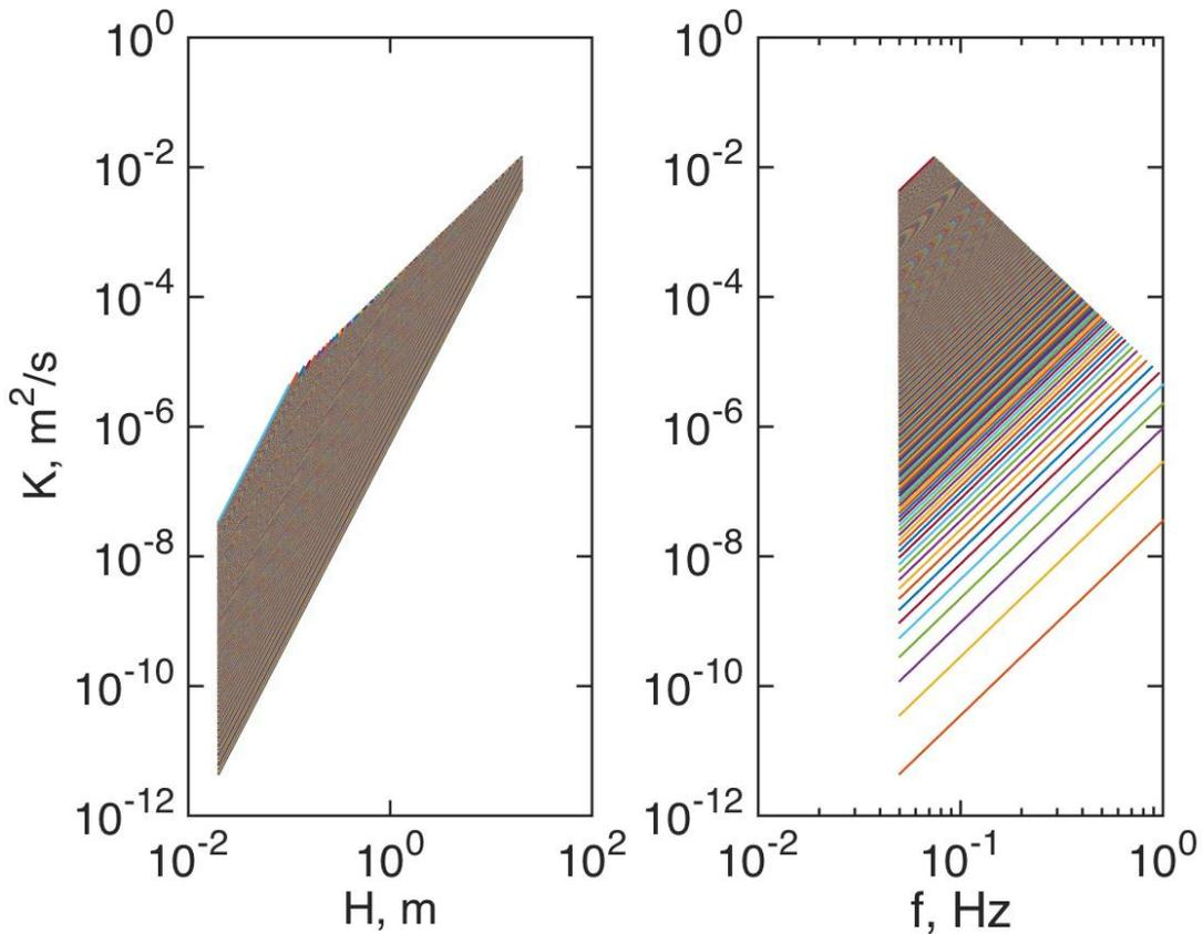
Fig. 1. Dependence of the coefficient of turbulent viscosity on (left) wave height for frequency  $f=0.05-1$  Hz; (right) frequency for wave heights  $H=0.02-20$  m
