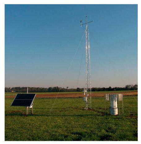
FIG. 3. A mesonet station in Kentucky with good exposure.
