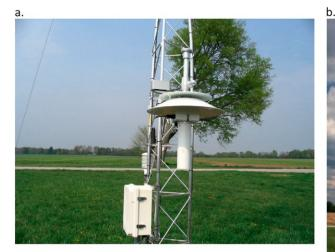
FIG. 4. (a) Aspirated radiation shield and (b) Gill radiation shield (naturally ventilated).
