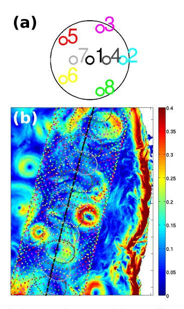
Figure 6. (a) Pattern of beams (1 is nadir, 4 and 7 are at 6°, the others at 12° incidence). The different colors help associating the footprint patterns in (b) with each beam. Background colors in (b) represent simulated currents velocities off the Oregon coast (in m/s), courtesy of Y. Chao, previously used by Fu and Ubelmann (2014) for the evaluation of the SWOT mission performance.
