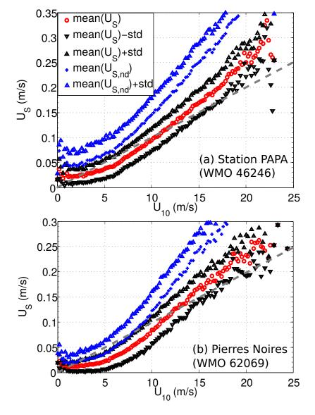
Figure 4. Example of mean value (in red) of the Stokes drift vector norm  $U_S = |(U_S, V_S)|$  as a function of wind speed for two locations: station PAPA in the North-East Pacific, and buoy 62069 off the French Atlantic coast. The black symbols show the mean plus or minus one standard deviation for each wind speed. The dashed grey line is  $U_S = 0.01U_{10}$ . For both buoys, the non-directional Stokes drift (in blue) is about 50% higher.
