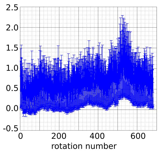
**Figure B1.** Maxximum velocity residual error (in cm/s) for the Oregon coast simulations. The Doppler centroid has been estimated for a fixed SKIM track over Oregon area. All WW3 run times of month 2014/09 are considered.
