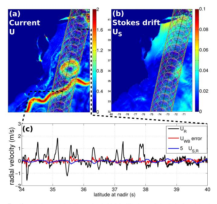
Figure A2. Example of (a) current in the Gulf Stream and associated (b) Stokes drift, and (c) errors for the estimation of UWB for beam 8  $(12^{\circ})$  incidence, green circles in top panels). In this example the standard deviation of err<sub>WB</sub> given by eq. (A6) is 10 cm/s, which is of the order of  $5U_{S,R}$ . Note that the measured geophysical Doppler is  $U_{GD} = U_{WB} + GU_{S,R}$  with  $G \simeq 25$ .
