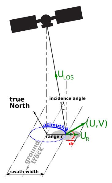
Figure 2. Geometry of measurement from a radar with a local incidence angle  $\theta_i$ , looking towards azimuth  $\theta$ . For simplicity of the schematic, we have taken  $U_{\rm WB}=0$  and  $U_{\rm NG}=0$ , so that the line of sight velocity is simply  $U_{\rm LOS}=(U\sin\theta+V\cos\theta)\sin\theta_i$ . Note that the diameter of the footprint (6 km) is exaggerated compared to the swath width (270 km) for readability.
