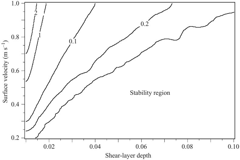
FIGURE 2. Maximum imaginary eigenvalue of the perturbation at time  $t = 0$  for a given shear flow of exponential type. For the stable region, all eigenvalues have null positive imaginary part up to computing accuracy.
