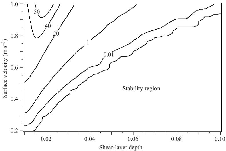
FIGURE 3. Maximum growth rate of an initial perturbation at time  $t = 0$  for a given shear flow of exponential type.
