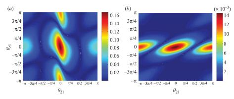
FIGURE 2. Dimensionless growth rate  $\alpha_r (b\sqrt{g/h^5})^{-1}$  as a function of  $\theta_{21}$  and  $\theta_{r1}$  for: (a) subharmonic and (b) superharmonic resonance; for fixed  $k_1h = 3.13$ ,  $k_2h = 2.06$  (therefore  $k_rh = 0.364$ ).
