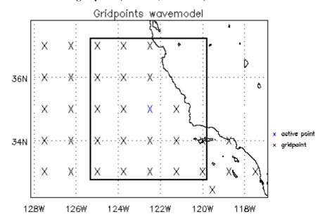
Nearshore location of buoy ndbc\_46053 on the west coast of the US at (34°14′10″N,119°51′00″W) with seaward normal at 205° and 417m water depth.
